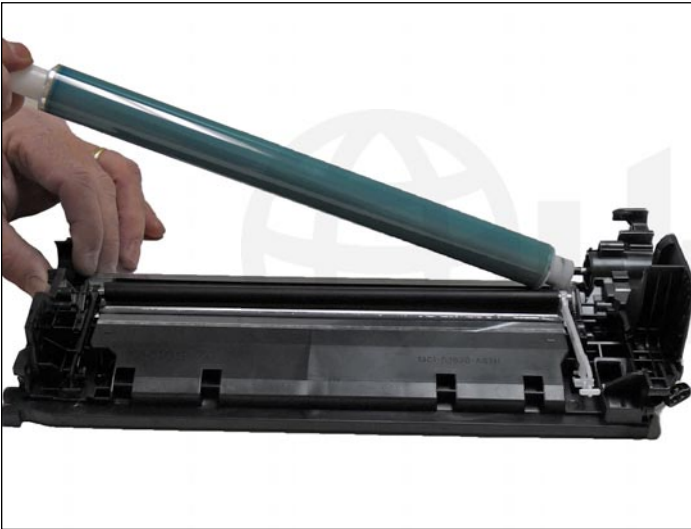
8. Remove the drum.
