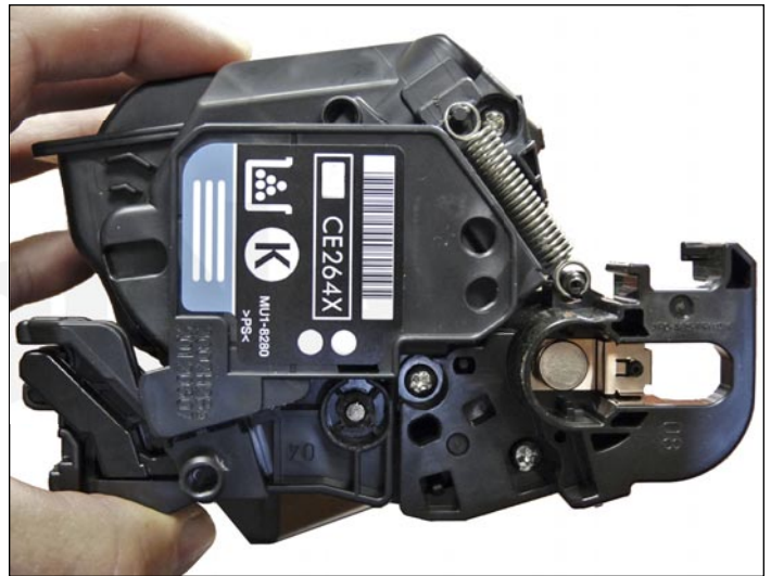
47. Install the spring.
