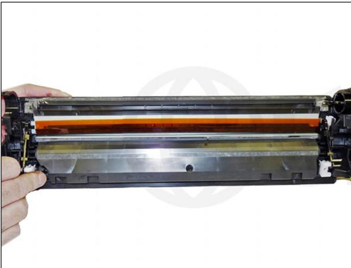
14. The amber film assembly is held in place with double-sided tape. If this is not sticking or a new wiper blade is being used, replace the tape. Replace the film assembly.
