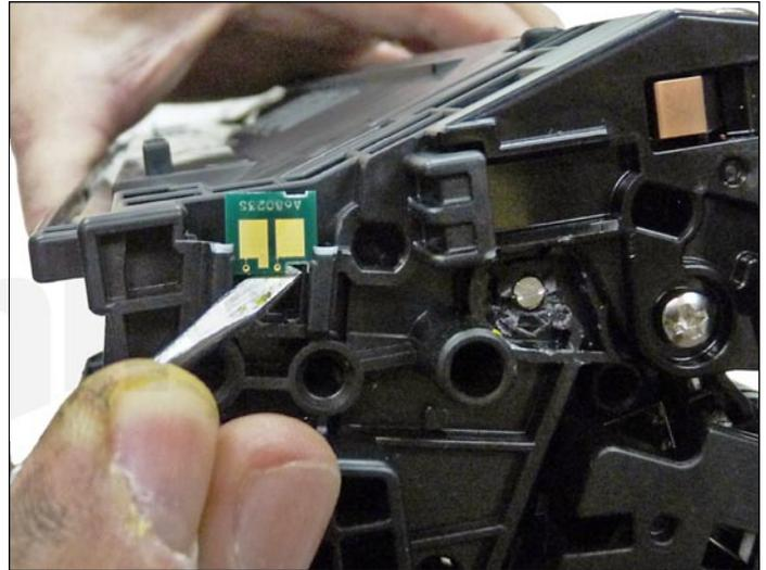
51. If the new replacement chip is loose in the slot.
