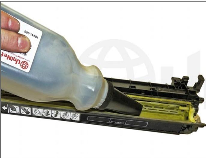
34. Clean out the remaining toner and fill with the correct color of toner for use in the HP M775 cartridge.
