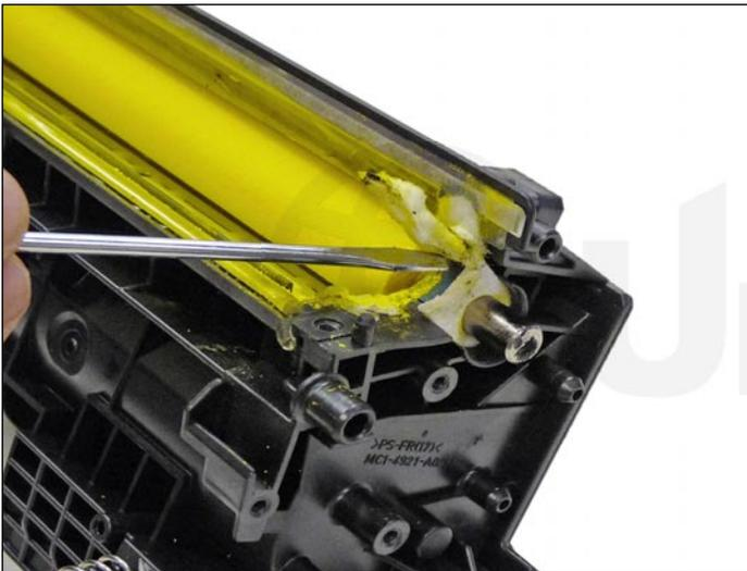
30. On the right side of the chamber, lift up the developer-roller felt seal. Lift it from the front side and lay it over the back.
