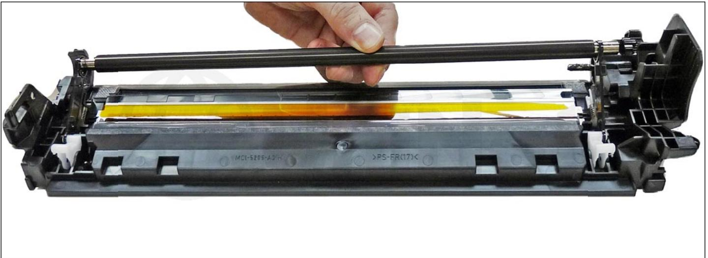
8. Remove the primary charge roller by lifting up on the black and white locking arms.
