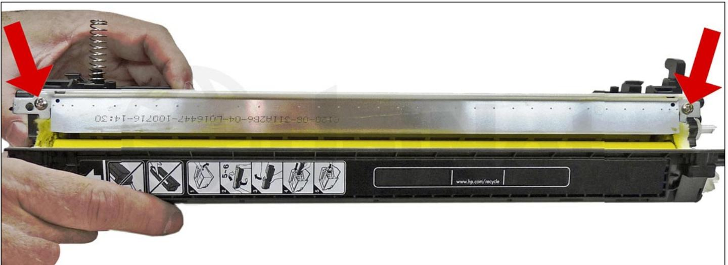
29. Remove the two screws from the doctor blade and start to lift the blade up.
