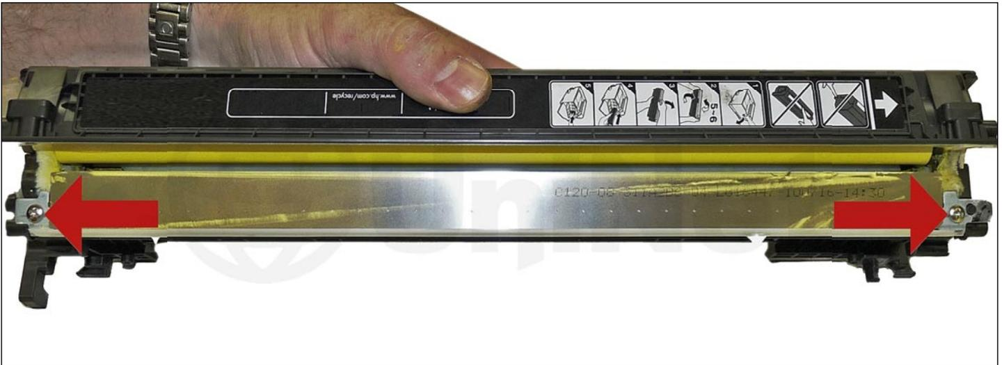
Install the doctor blade and two screws.
