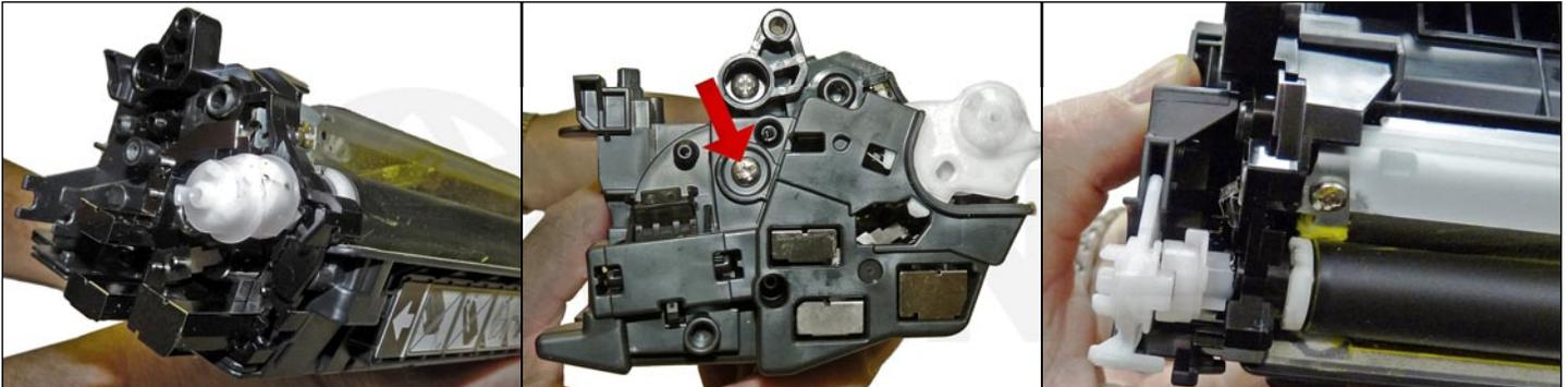
46. Place the triple gear on the developer roller shaft and fit into the spring assembly on the end cap.
