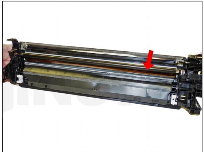
15. Clean the primary charge roller (PCR) with your preferred cleaner and install in the cartridge with the PCR holders. Make sure you lock the locking arms in place.
