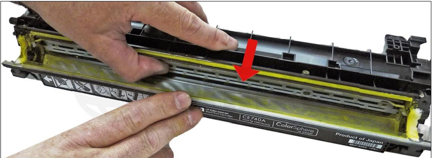
Install the seal onto the seal rails. Pull the release tape off 1" at a time and press the seal in place as you go.
