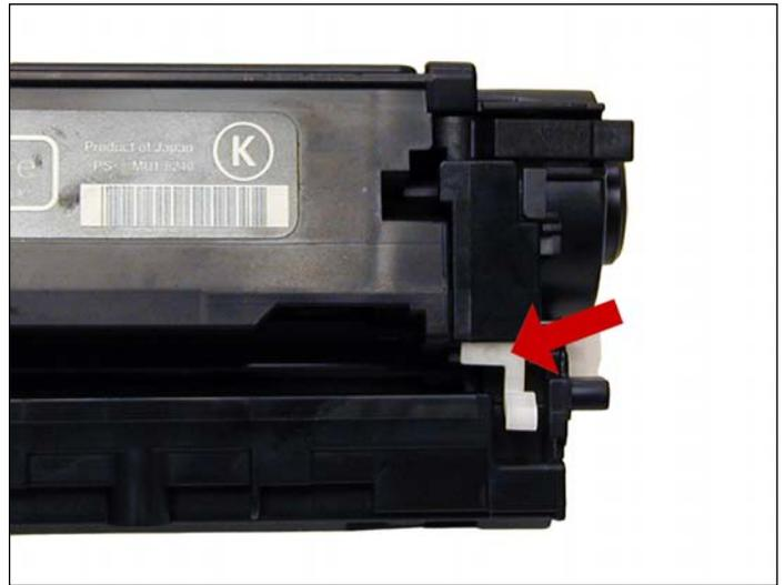
26. Hold the two halves together. Align the spring on one side and the spring loaded arm on the other.
