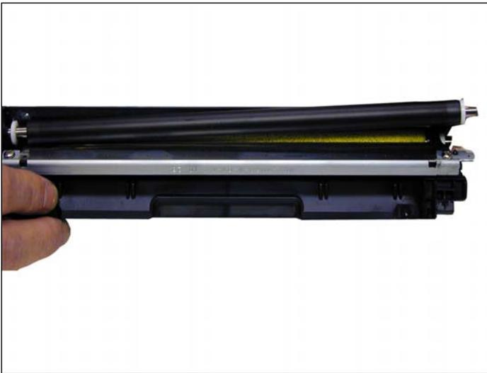
12. Slide the developer roller over and remove.
