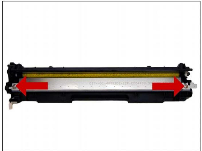
13. Remove the two screws and doctor blade.
