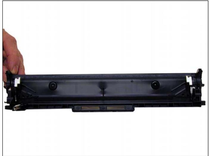
5. Remove the two screws and wiper blade.
