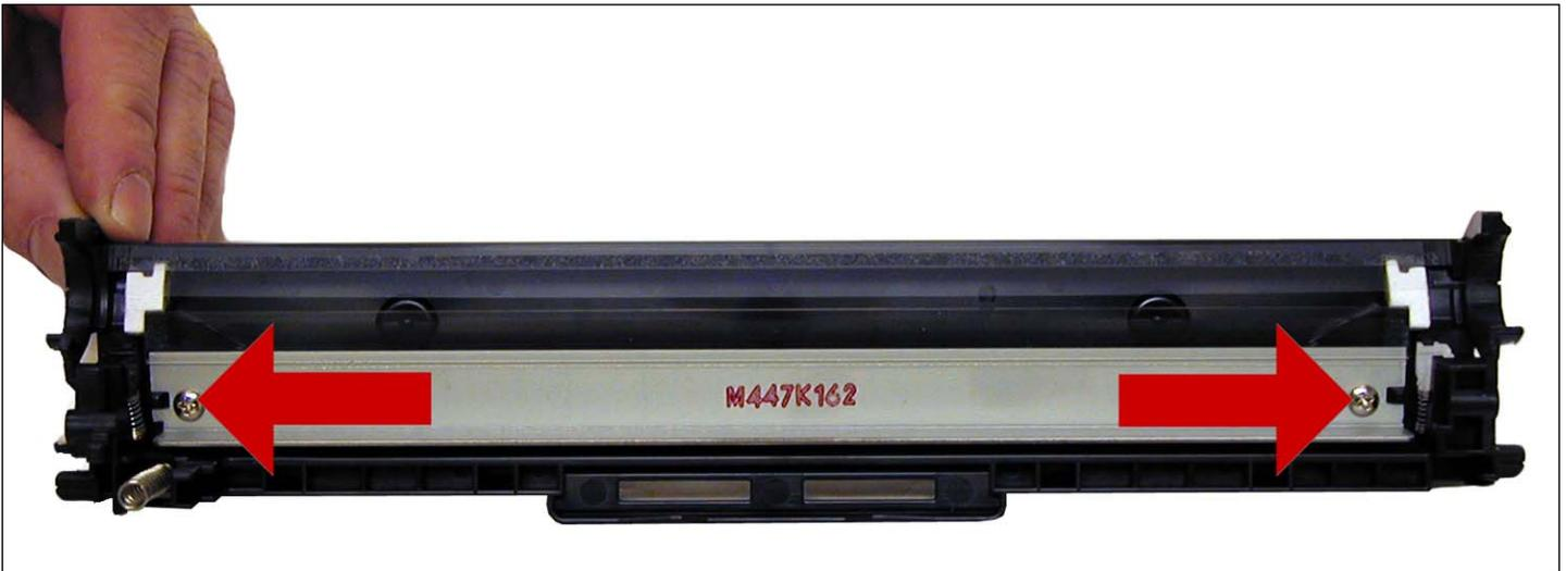
7. Coat the new wiper blade with your preferred lubricant and install. Install the two screws.
