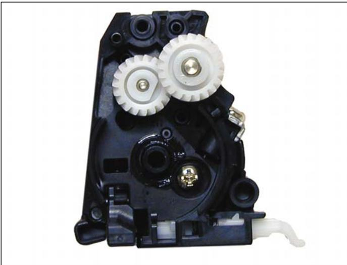
23. Replace the 2 gears on the feed and developer roller shafts.
