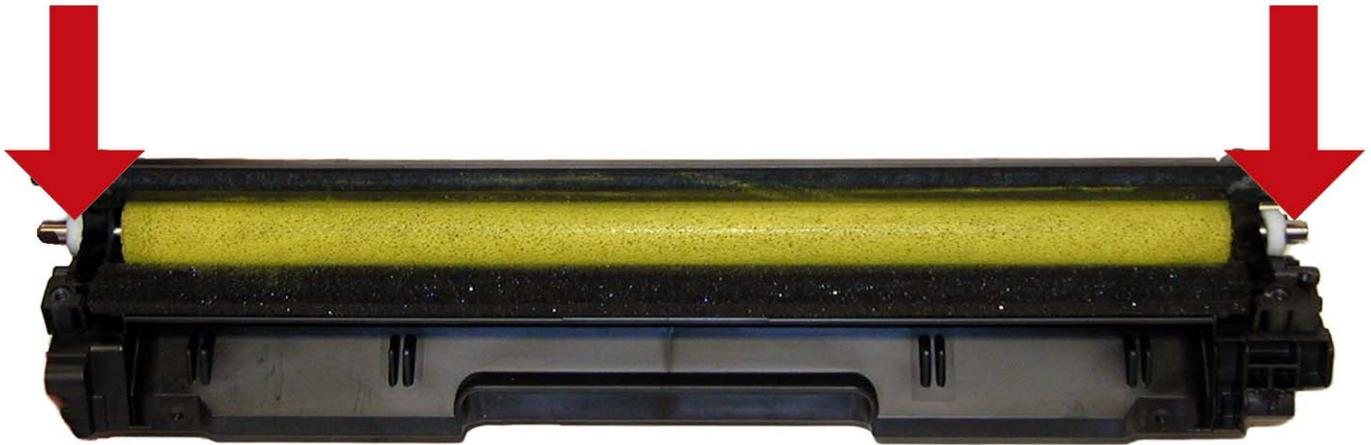
17. Install the two white felt seals on the feed roller shaft.
