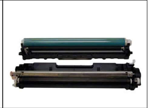
2. On the right side, remove the two screws and end cap.
