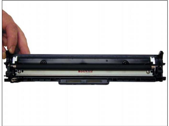
8. Install the cleaned PCR. Make sure to place a small amount of conductive grease on the black PCR holder.
