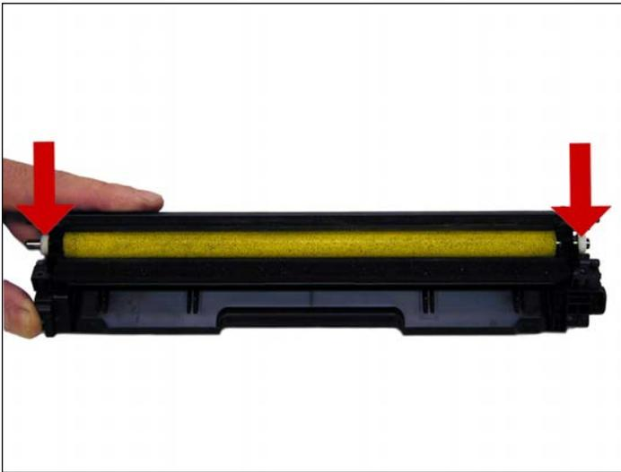
**NOTE:** HP/Canon created a bit of a block for us here. The clear bushing located on the right side of the hopper (pictured) is glued in. The opposite side bushing is integral to the hopper. If you wish to install a seal, change the feed roller, or just have better access to the hopper, the feed roller must be pulled over to one side compressing the foam.
