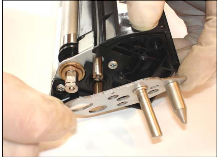
14. Release the metal gear endplate.
