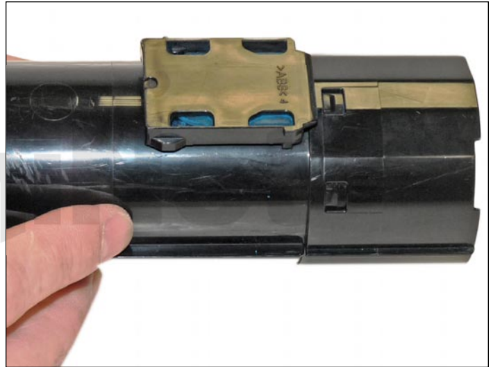
4. Open the toner port and clean out any remaining toner.
