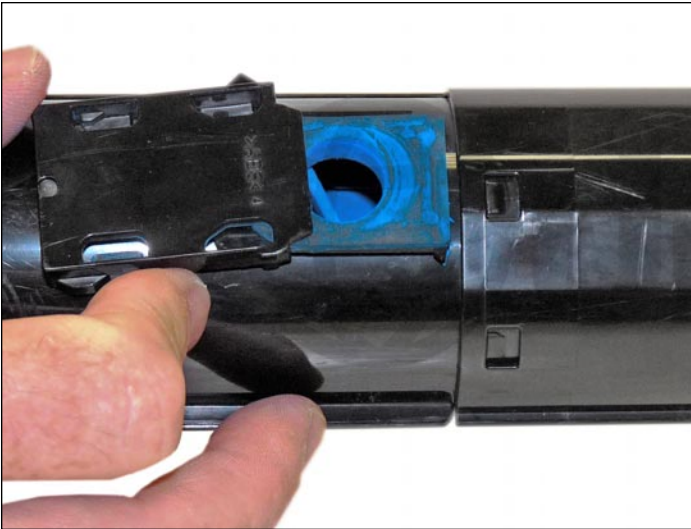
4. Open the toner port and clean out any remaining toner.
