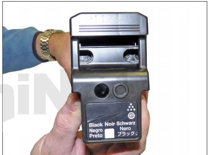
7. Install the end cap on the cartridge. An easy way to do this is to place four drops of hot glue on the four broken posts. Quickly place the end cap on before the glue dries. If further help is necessary to keep the end cap on, black tape along the seam works well.
