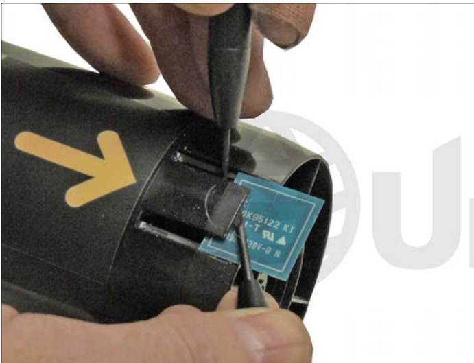
5. Replace the chip by prying up the center tab while using a small screwdriver to move the chip out.
