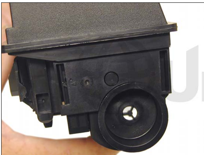
3. Re-install the fill plug.
