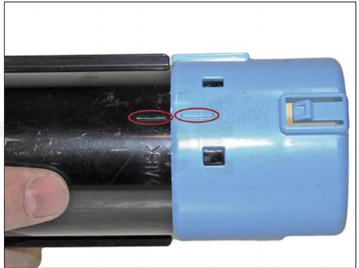
6. Align the two marks on the end cap and tube.
