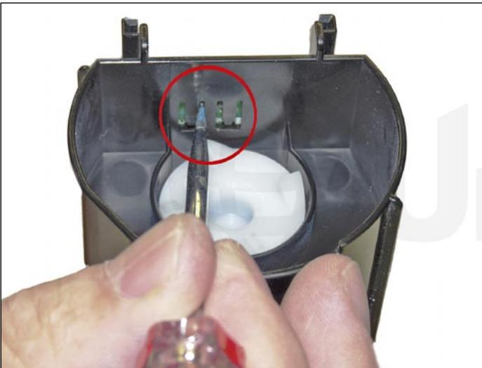
7. Using a small Jeweler's type screwdriver, pry up the chip through the small slots underneath and slide it out.
