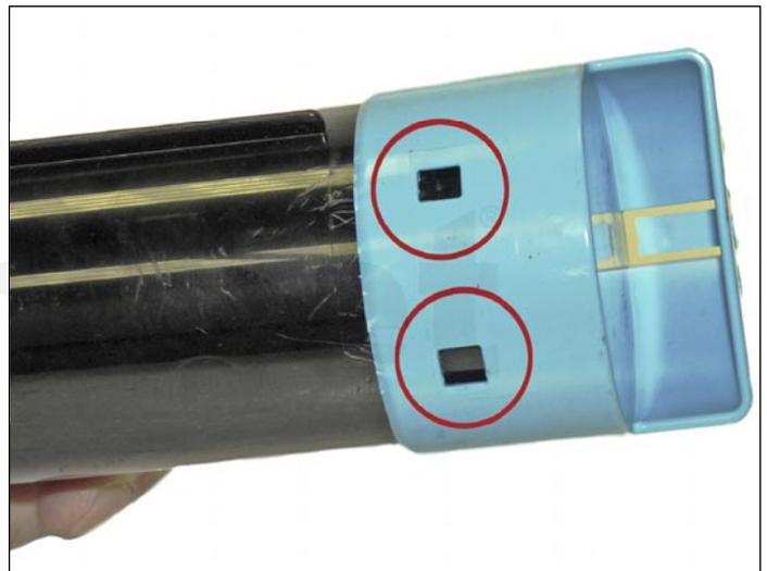
1. Pry up on the colored end cap by lifting up all four tabs.
