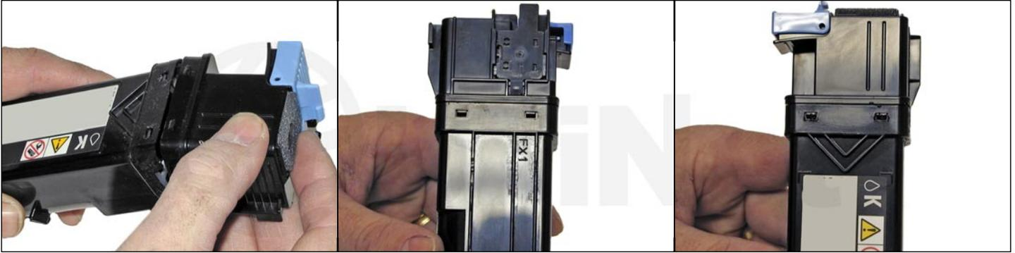
6. Install the waste chamber on to the supply hopper.
