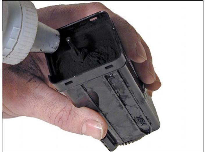
4. Fill the hopper with toner for use in the Dell 2130/2135. Remember, while the cartridges all look the same, they are not interchangeable. Each color has a different set of plastic tabs.
