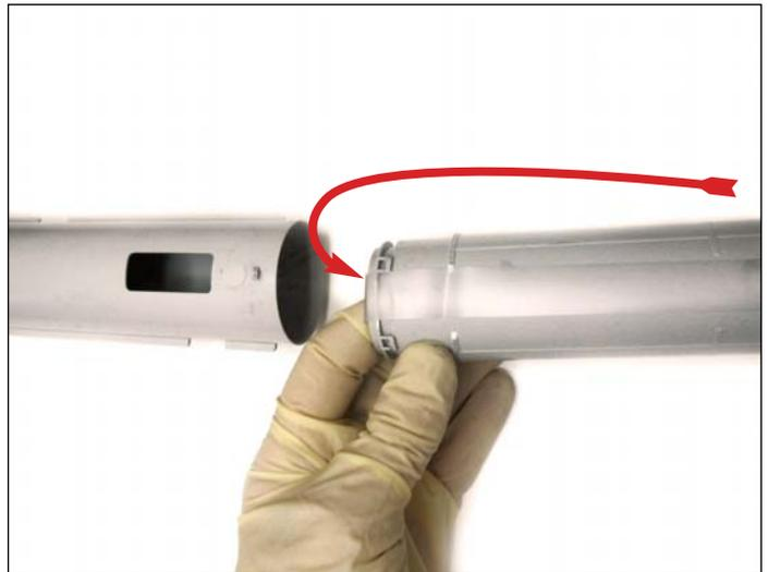
14. Gently wrap the seal flap around the toner fill opening (as shown) while you prepare to insert the cartridge. This will ensure that the seal flap properly exits the opposite end of the container.
