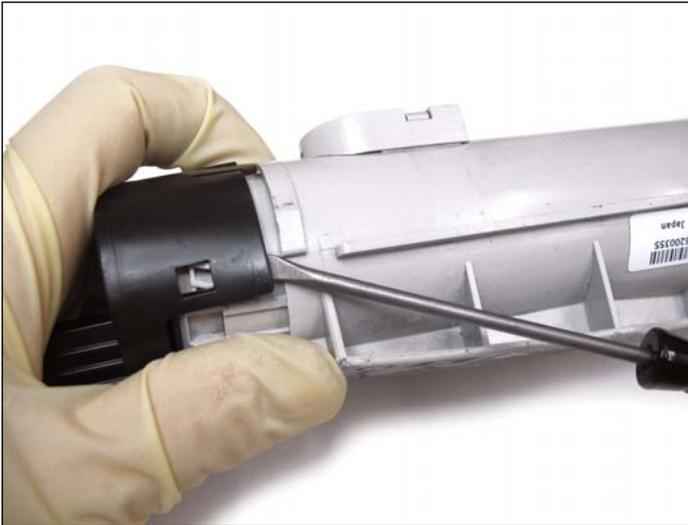
2. Rotate the cartridge and disengage the third tab (shown) in the same manner.
