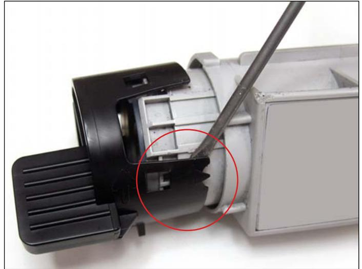
3. Disengage the fourth tab as shown.
