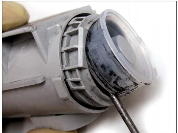
6. Carefully lift the toner fill plug out as shown. Be careful not to damage the plastic housing.
