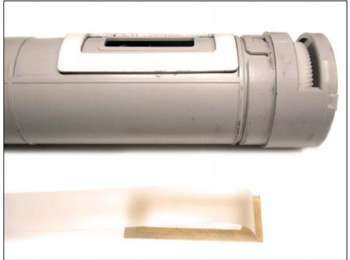
**INSTALLING THE CLEARSEAL™ ADHESIVE**
