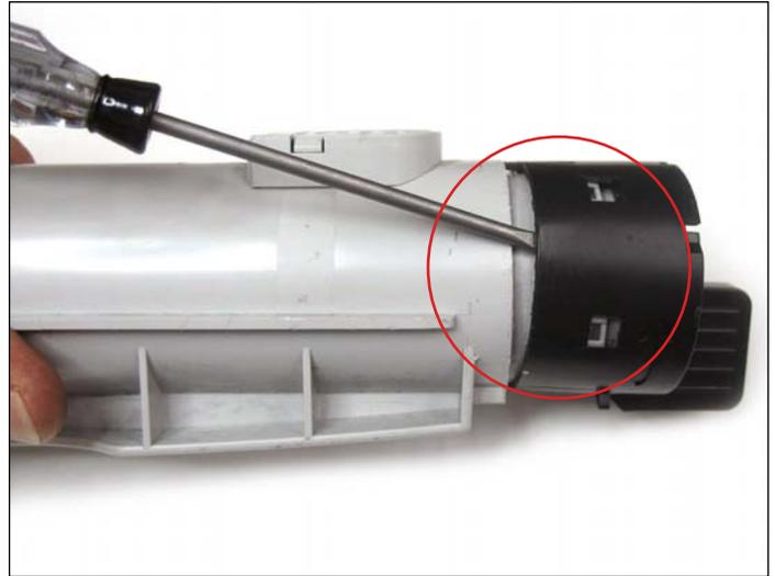
**REMOVING THE GEARLESS END CAP**
