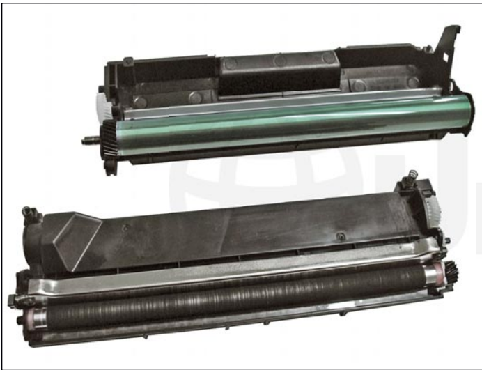
5. Lift off the waste chamber.
