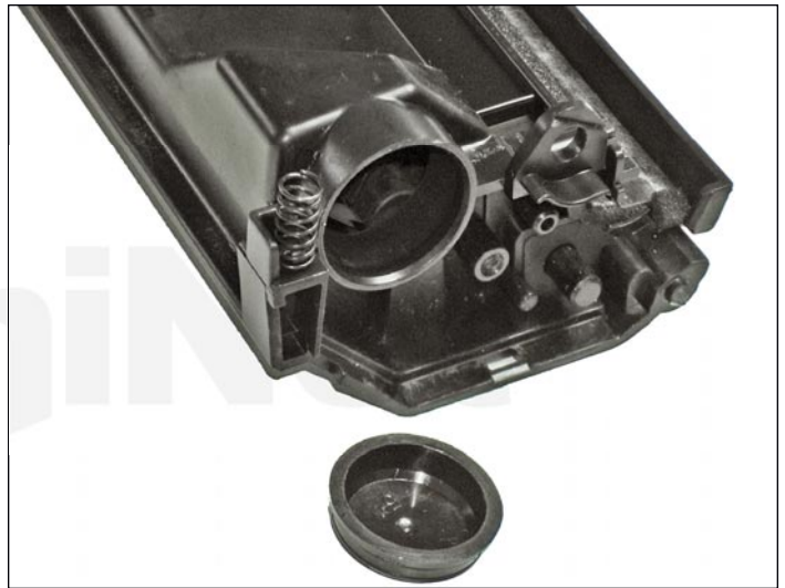
15. Carefully pry out the fill plug, as it fits tight and can be easily damaged. Work a small jeweler's screwdriver around the edge until the plug comes free.
