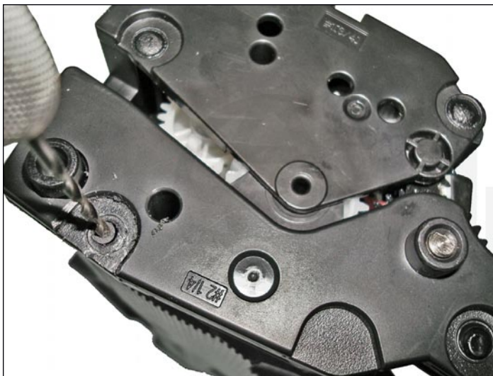
26. Drill holes where the plastic rivets were and install the screws.
