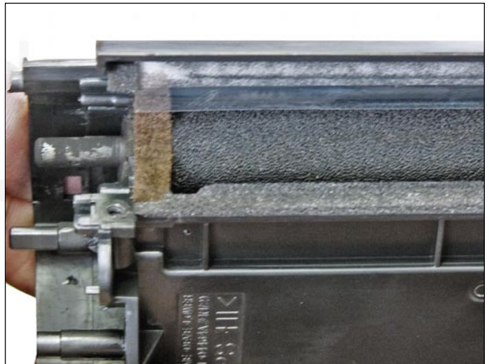
18. Clean the feed roller and any remaining toner from the hopper.
