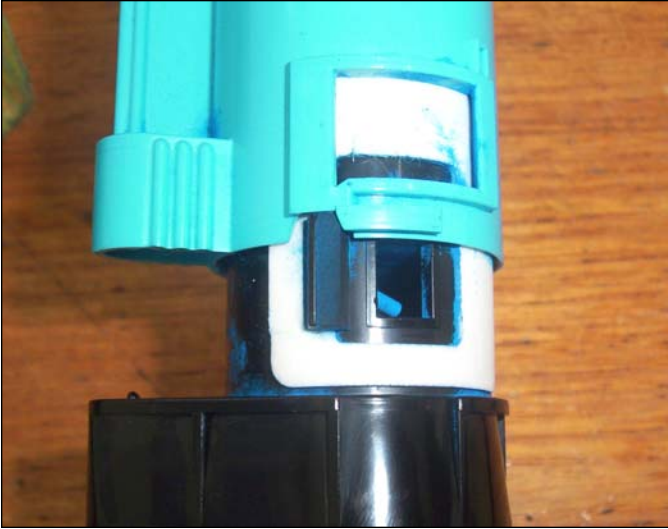
5. Now pull the cap, out away from the cartridge.
