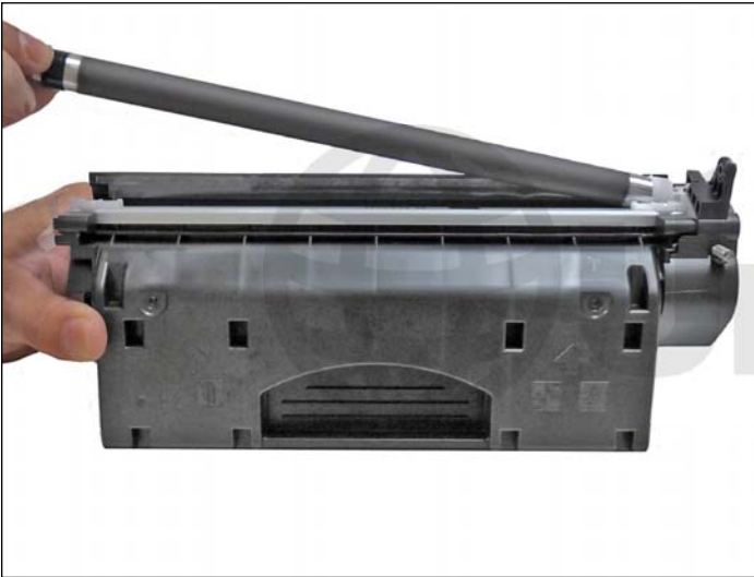
15. Remove the magnetic roller assembly.
