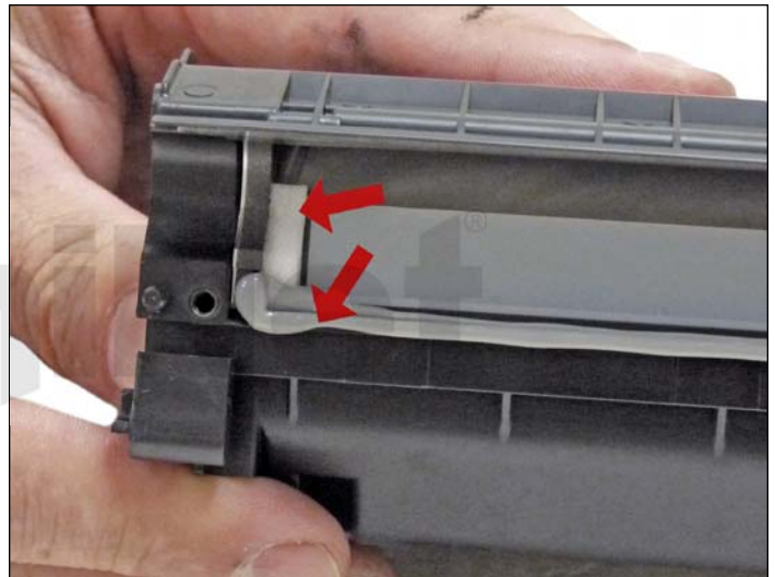
18. Clean out any remaining toner from the hopper. Note the doctor blade seal. It is a sticky substance that can be clean with alcohol if toner gets on it.
