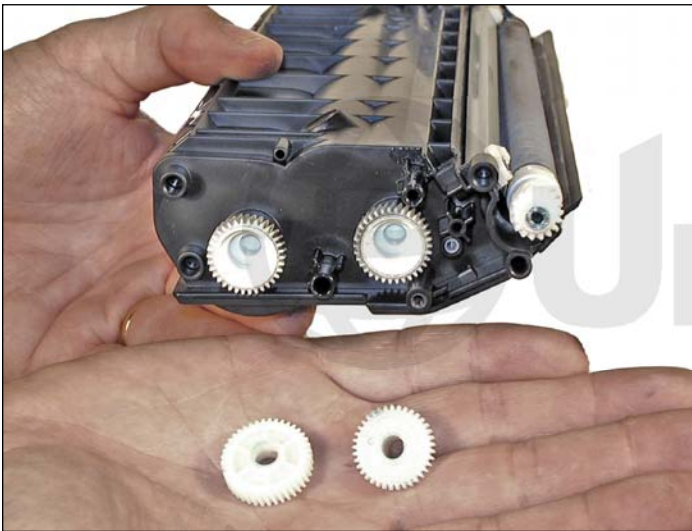
16. Remove the two gears as indicated. The remaining two gears should not be removed. They will not fall off, and are mounted to the toner augers inside the hopper.
