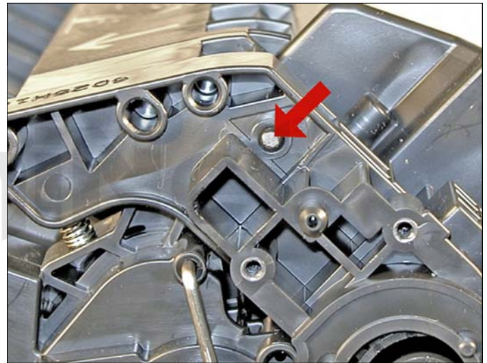
29. Place the two halves together, making sure the arms on the toner hopper are aligned and insert the two pins.
