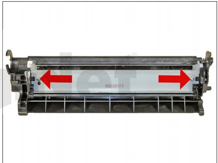
9. Remove the two screws and wiper blade.
