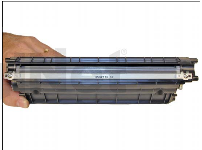
19. Remove the two screws and doctor blade. Pry the blade up from the right side. There is adhesive under the blade. If you pull the blade off, the alignment pin may break off.
