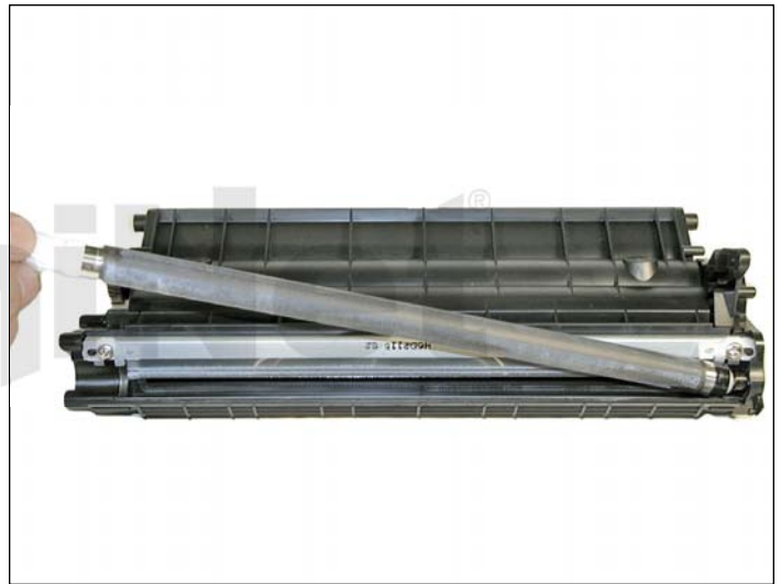
17. Remove the magnetic roller assembly.
