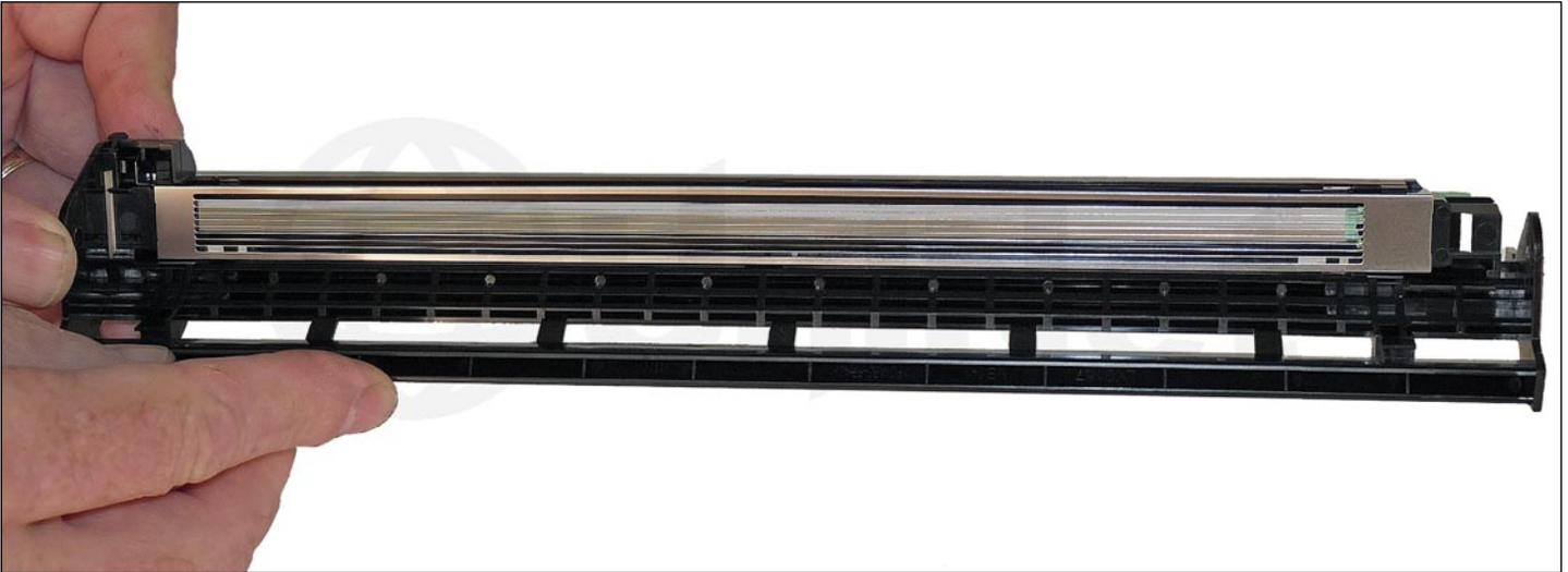
10. Install the drum (gear side to the right).
