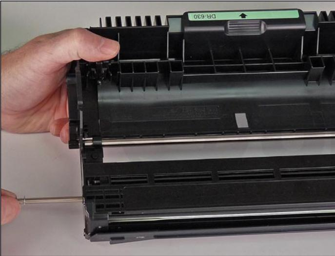
13. Install the drum axle from the left side.
