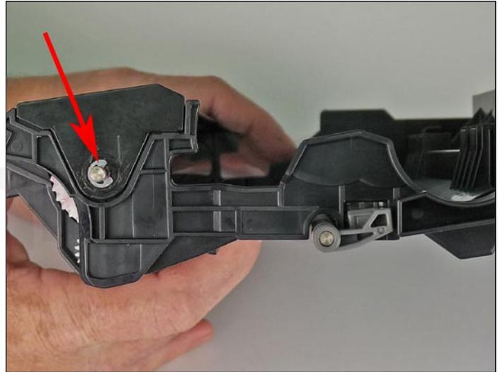
14. Install the "E" ring onto the axle.
