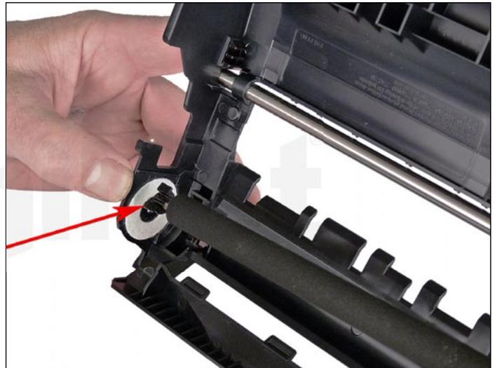
6. Remove the Transfer Roller from the cartridge.
