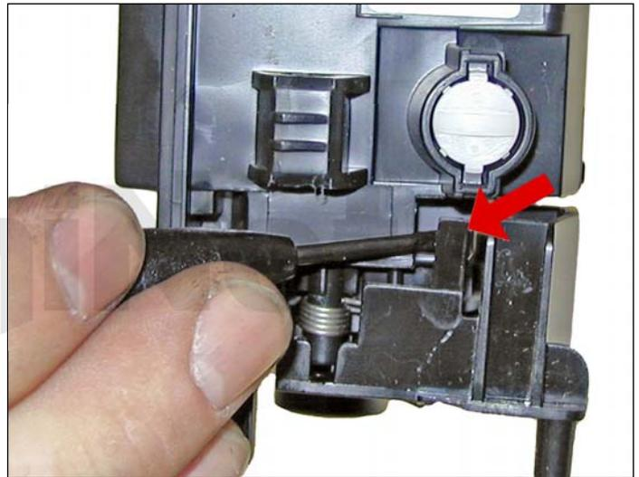
5. Lift up on the tab indicated and remove the end cap.
