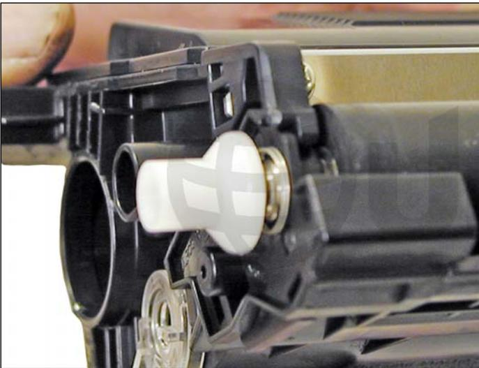
16. Install the spring and bushing on the non gear side of the roller. Make sure the bushing moves freely.
