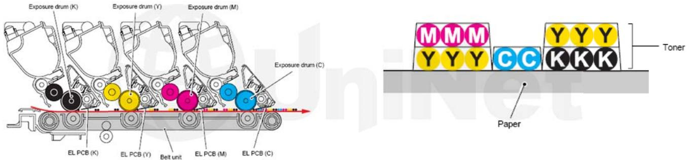
The **fourth stage** is the transfer stage. In the transfer stage the transfer roller which is located directly opposite each OPC drum, places a positive DC bias charge on the back of the Image Transfer Belt. Each toner cartridge has a separate transfer charge roller. The image is transferred from the drum directly to the paper. This process is repeated for each color cartridge in the following order: Black, Yellow, Magenta and Cyan (see left image).
