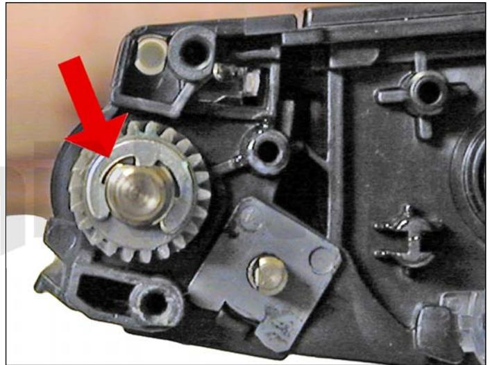
7. Remove the E-ring and developer roller gear.
