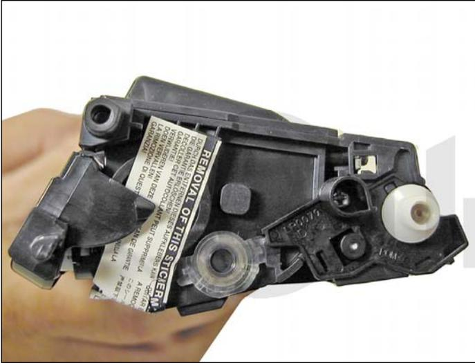
1. Vacuum the exterior of the cartridge. Be careful not to damage the developer roller as it is exposed.
