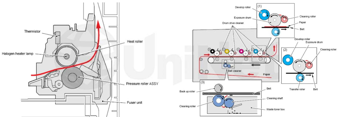
In the **fifth stage**, the image is then fused onto the paper by the fuser assembly. The fuser Assembly is comprised of the upper heating roller and lower pressure roller. The lower pressure roller presses the page up into the upper heating roller which then melts the toner into the paper. This heating assembly consists of a hard metal coated roller with a halogen lamp inside.
