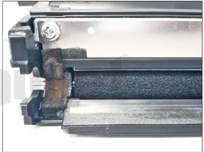
13. Vacuum/blow the doctor blade. We do not recommend that the doctor blade be removed as the developer roller felt seals will be disturbed. Once a new blade is available, great care will have to be taken not to tear the seals causing a leak. The doctor blade can be easily cleaned by blowing the excess toner off, and wiping down with a lint free cloth. Be very careful not to leave any lint behind and do not use any chemicals to clean it!
