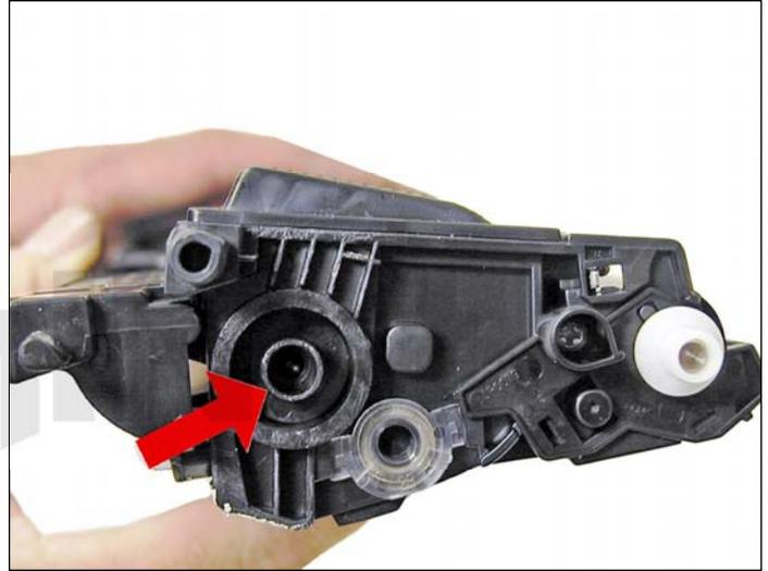
2. Remove the fill plug from the toner cartridge. Dump the remaining toner and vacuum/blow out the cartridge. There will probably be a label over the fill plug. It comes off with a little alcohol and a lint free cloth or cotton swab.
