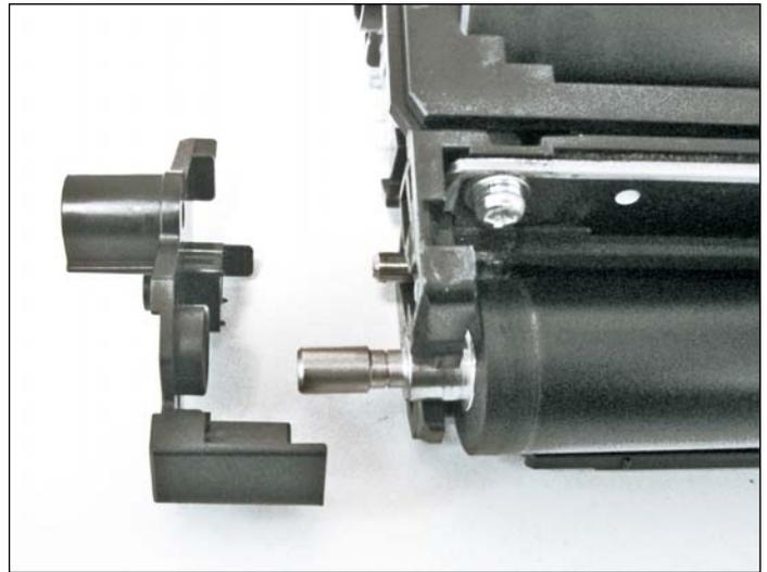
9. Lift the tab shown to release the developer roller support.
