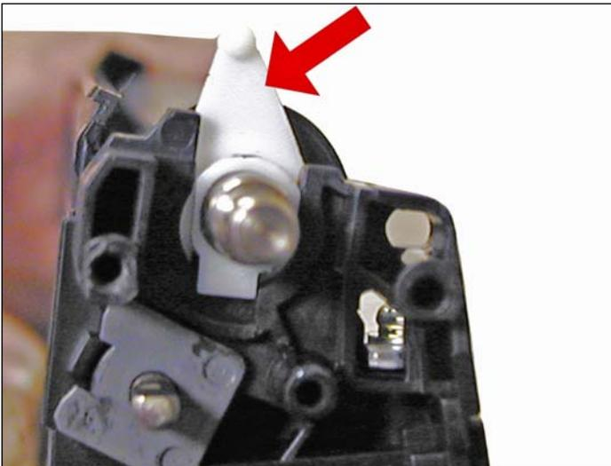
10. Move the white plastic locking tab on the right side of the developer roller to the "up" position.
