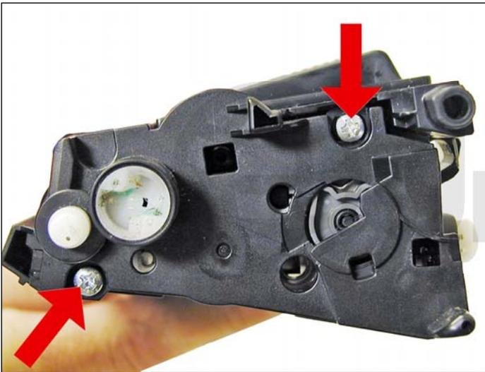
4. With the handle facing you, remove the two screws on the left end cap.
