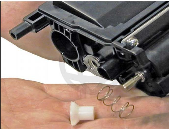
8. Gently pry off the white bushing on the opposite side of the developer roller. Be careful not to lose the spring!
