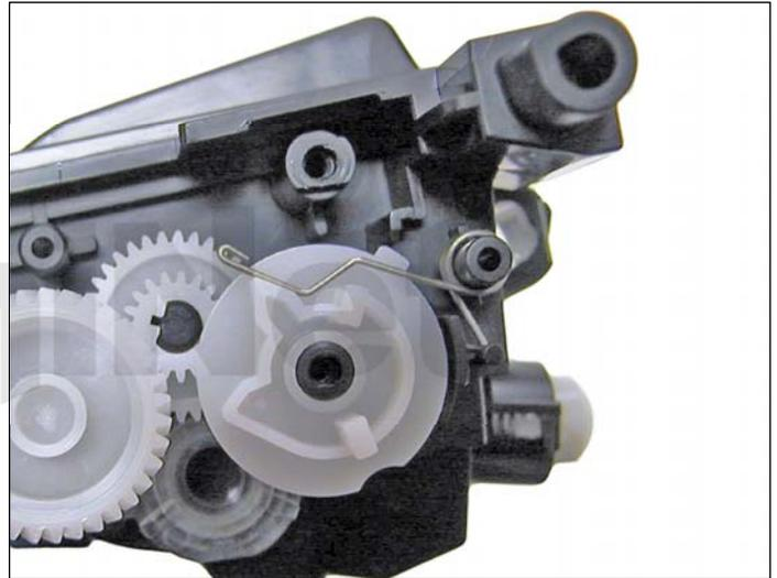
19. Set the reset gear and spring as shown. The tail of the spring fits into a notch at the base of the gear.
