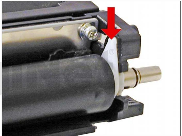
15. Install the cleaned developer roller, long-shaft side to the gear side, and white lock pointing up.
