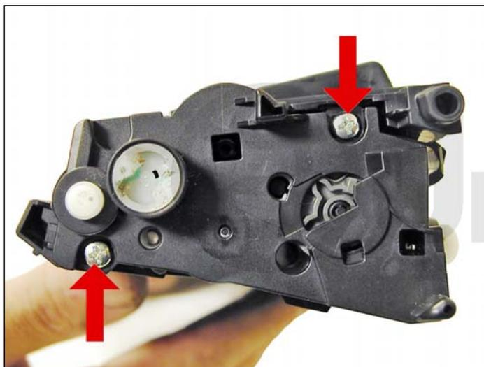
20. Install the gear cover plate, and two screws.
