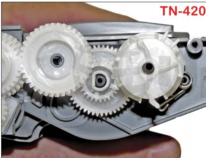
19. Depending on the cartridge you have, set the reset gears as shown for the TN420 (left image) and TN450 (right image).
