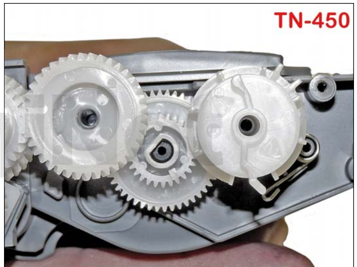
19. Depending on the cartridge you have, set the reset gears as shown for the TN420 (left image) and TN450 (right image).
