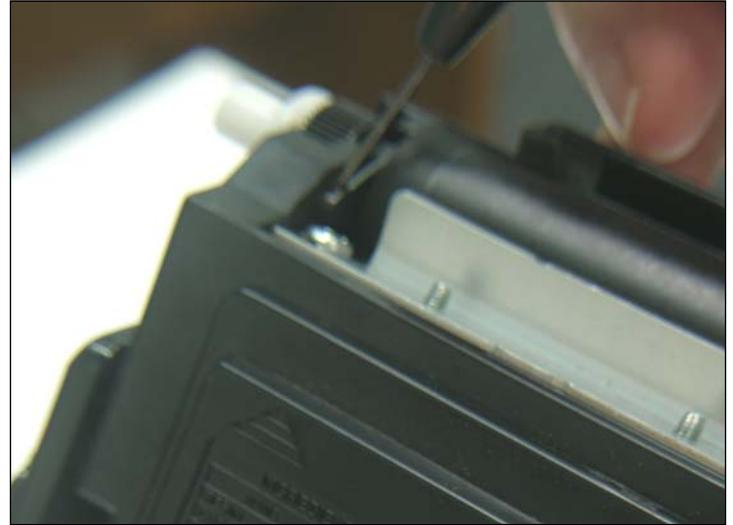
5. Move to the other side of the cartridge and above the white plastic hub on the gear side, locate the clip that holds the developer roller cap-bearing. NOTE: Contrary to the other bearing cap this one is located between the developer roller and the side of the cartridge.
