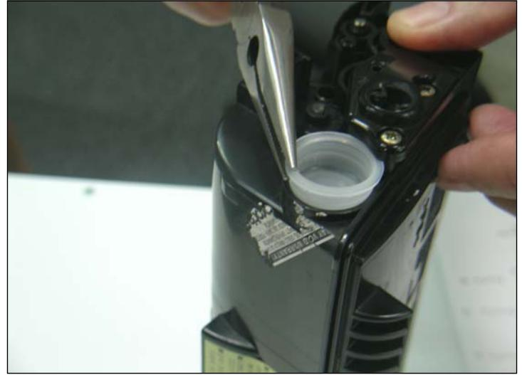
8. Remove the fill plug from the hopper. Discharge any toner from the toner hopper. Use dry compressed air or a vacuum to THOROUGHLY clean out the toner hopper. Clean the developer blade using a dry lint free cloth.
