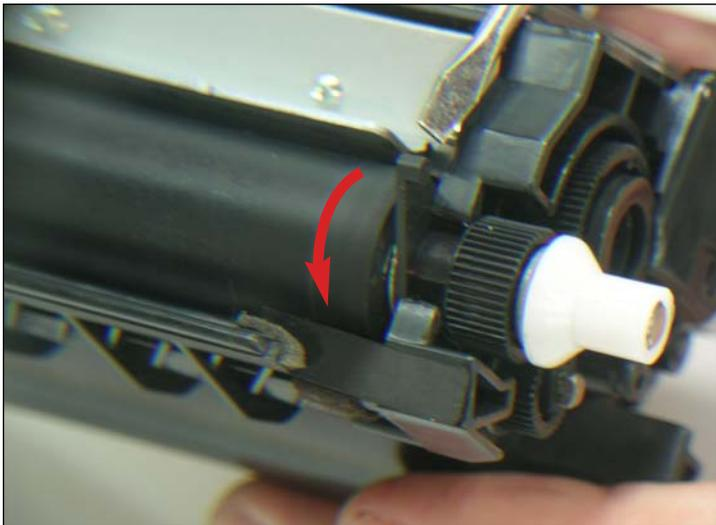
6. Press the clip in towards the developer roller and rotate the piece up towards the front of the toner hopper, until the bearing cap is perpendicular to the roller.
