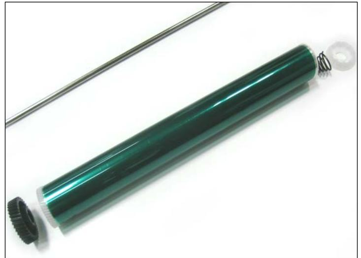
22. Do not lose these three pieces which will be needed to assemble the cartridge even if a new drum is installed.
