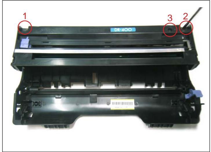
12. With a medium size Phillips screwdriver remove the screws securing the corona wire assembly. There are two in each corner holding the plastic top and one, visible thru the hole on the right hand side securing the electric contact of the control grid and the cleaning felt.
