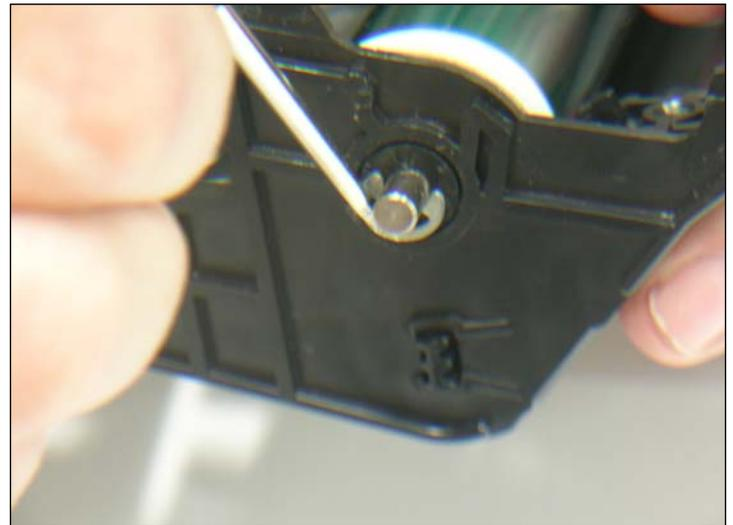
18. Remove the shaft of the drum by releasing the retaining washer from the left side of the cartridge.
