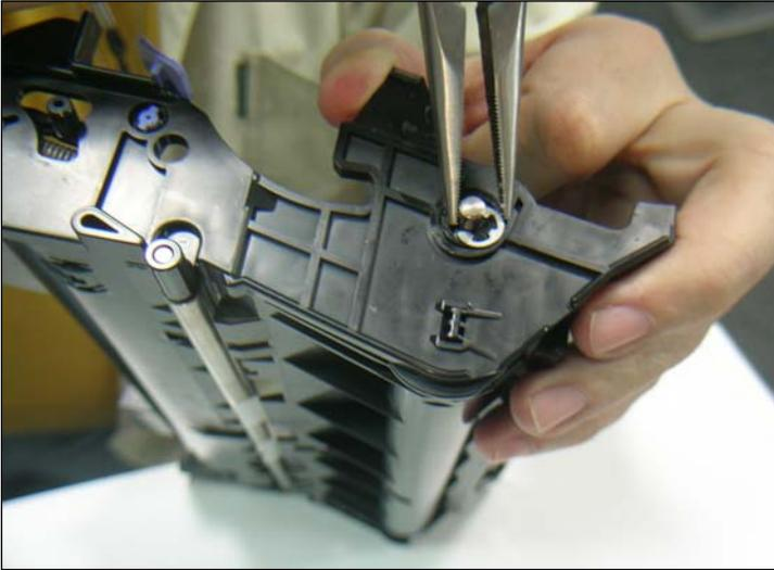
19. Pull axle out using a pair of needle-nose pliers.
