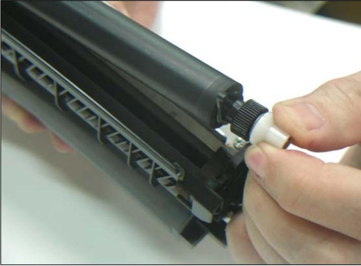
7. Lift the developer roller from the hopper. NOTE: Clean the roller using a clean lint free cloth. DO NOT USE any solvent or chemicals on the developer roller.
