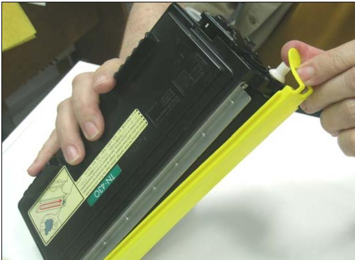
11. Insert the OEM or the compatible yellow seal cover for the developer roller to protect it during transit.
