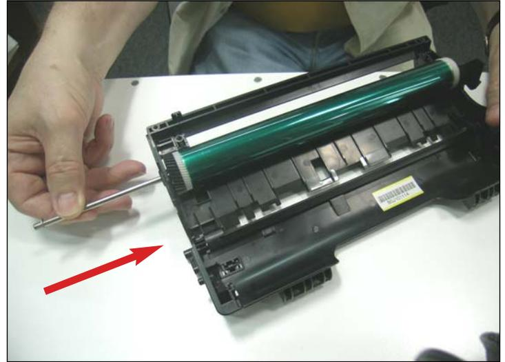
26. Slide the axle from left to right, insert the bearing in place and the retaining washer to secure the axle in place.
