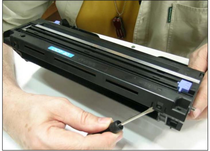
29. Insert the lid containing the corona assembly, align the four clips, and press down to clamp it.
