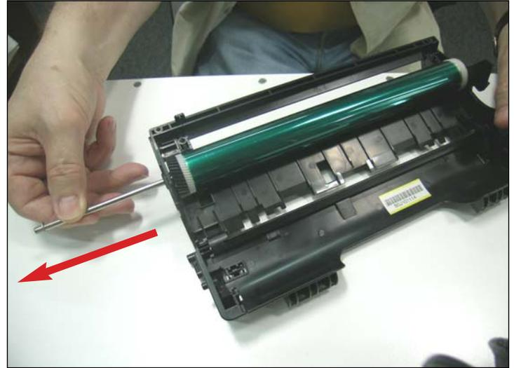
20. Slide the axle away from the cartridge as shown.
