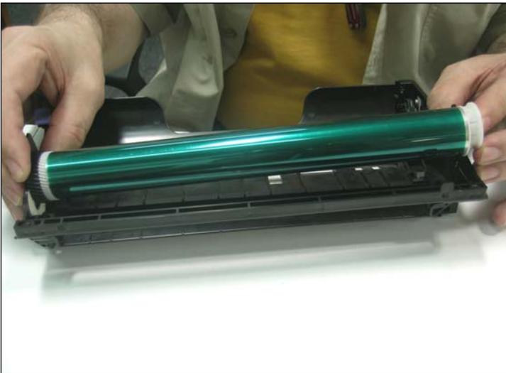
21. When the drum is extracted there will be a spring loaded clutch piece at one end and a drive gear on the other side coming loose.
