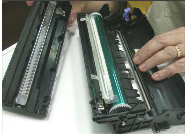
14. Clean the grid surface of any toner with compressed air.
