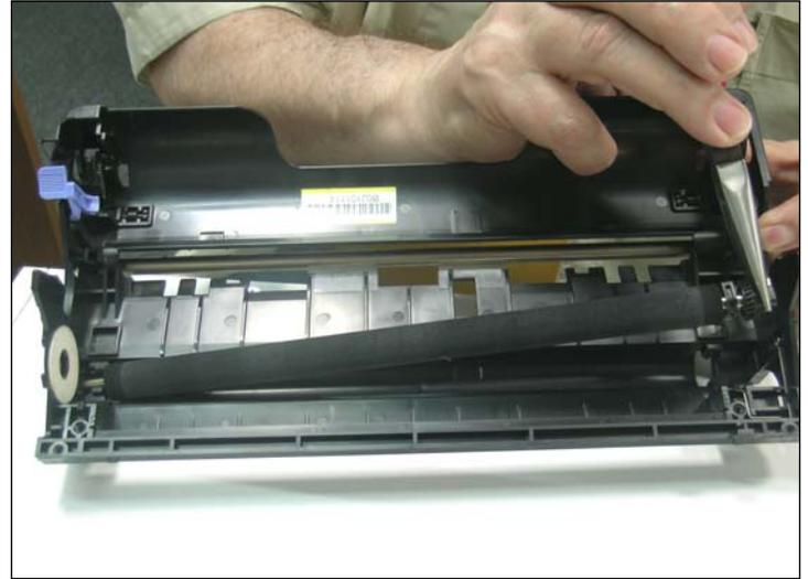
24. Extract the transfer roller from the cartridge using a pair of long nose pliers. Notice that the saddles and the helical gear will also come out. Clean the roller with compressed air or vacuum cleaner. DO NOT USE any solvent or chemicals on the transfer roller.
