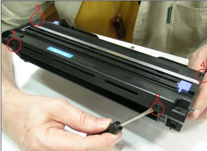
13. Press the four tabs to remove the assembly from the top of the cartridge starting from the two behind followed by the ones on each side.
