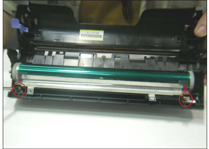
16. With a Phillips screwdriver remove the screws holding the drum cleaning assembly. You will notice that it is composed of a cleaning felt, a recovery blade and a couple of scraper-blades.
