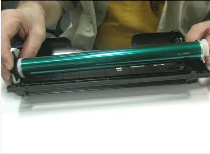
25. Replace the OPC drum by mounting the clutch and spring on the right side and engage the drive gear on the left.
