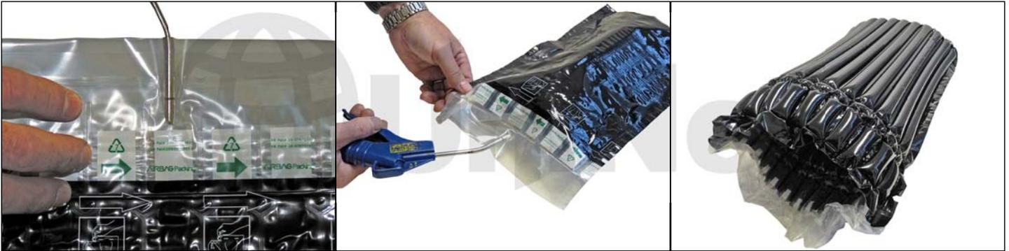
1. Inflate the bag by inserting the air gun nozzle into the center fill port of the bag as shown
